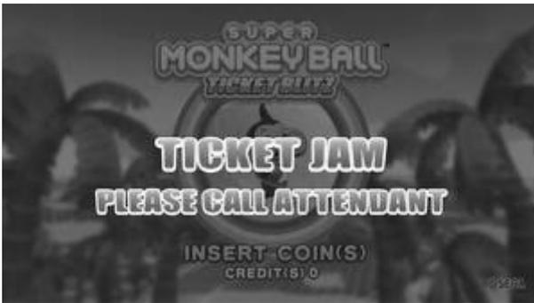
This message will appear when ticket(s) are jammed on TCIKET DISPENSER. Refer TICKET JAM action to remove jammed tickets(s) from TICKET DISPENSER. After remove jammed tickets then fill the tickets correctly then press RELEASE button to back normal.
